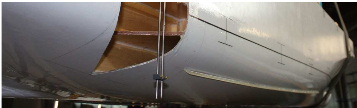
Figure 10: Bilge keel arrangement
